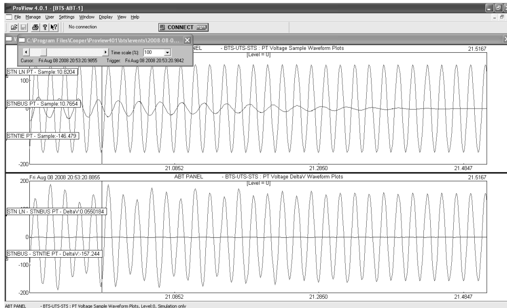
Fig. 2.2 : Voltage Waveform and Delta V Waveform for Station-to-Station Scheme – Note that Alternate Station Voltage is available and healthy.
